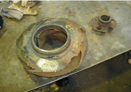
This is a Duplex Impeller after only 16 weeks in service.
