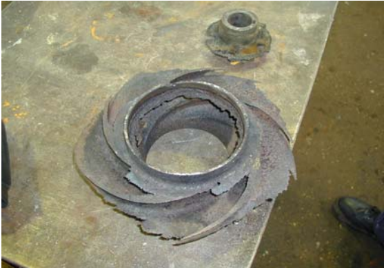
This is a 13% Chrome Impeller after only 12 weeks in service.
